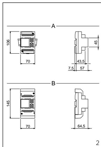
It can also be surface mounted, using the DIN rail supplied, but fitted with terminal covers. Dimensions are shown in figure 2B.
