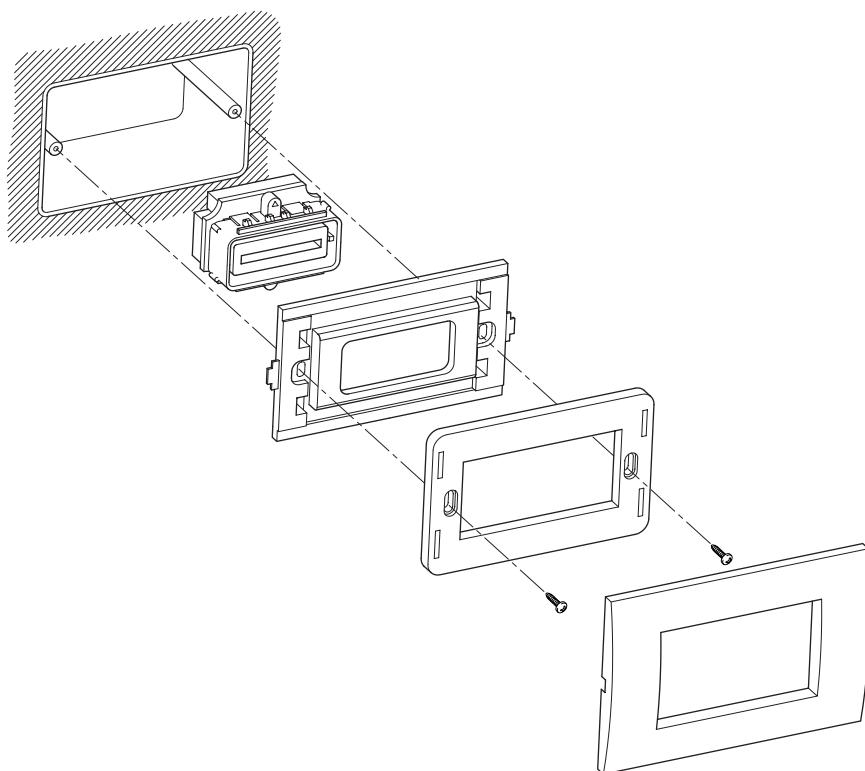
Fig. 1 - Mounting the socket in 3-module embedding box with BPT plate or compatible ones.
