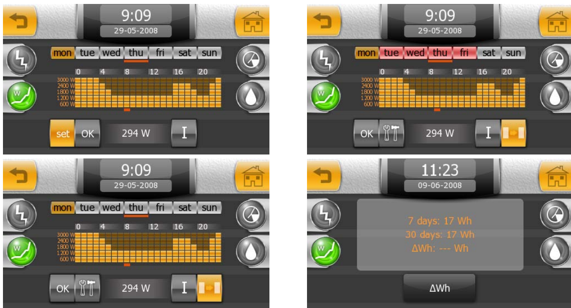
Example: check loads and consumption management with release priority list, 4 time periods with different priorities for each load.
